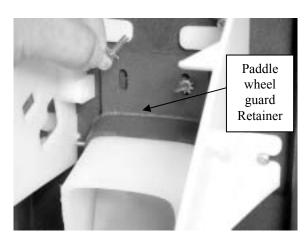
**8** Remove the two thumb screws from the plastic paddle wheel guard retainer.
